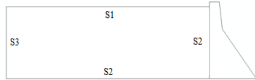
Fig1. Boundary conditions for the dam and reservoir
