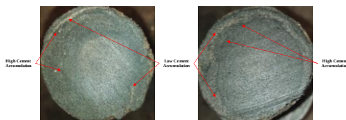
Fig. 2. Cross-sectional examples of DSM columns from the first group.
